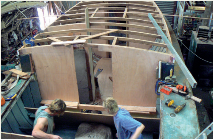
Above: Various stages of the deck rebuild and the relaunch at Michael Dennett Boat Builders - Neil was delighted with the work they did
